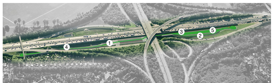
Reference sections: 1 longitudinal evenness, 2 transverse evenness, 3 skid resistance, 4 substance characteristics (surface), 5 texture
